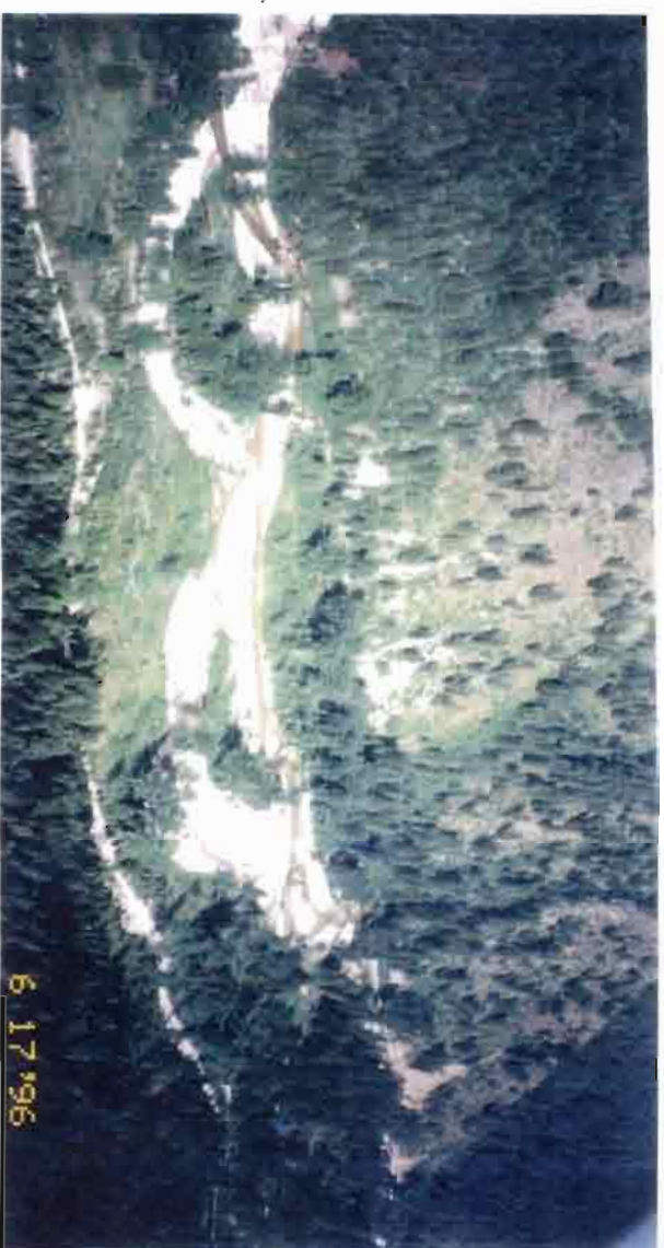
View of channel just upstream of Langlois Creek confluence. New channels were cut through riparian vegetation during floods of 1996.
