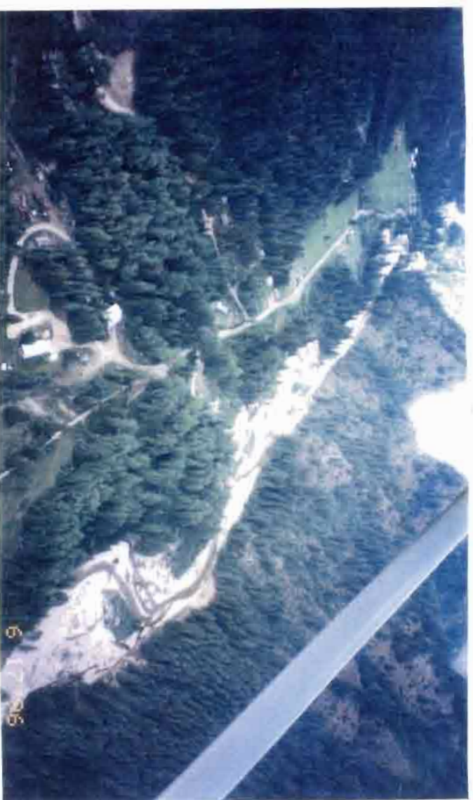
View downstream of the confluence of Langlois Creek and vicinity. Wide, shifting unstable channel occurs throughout this reach. One site of hillside erosion is visible where channel impinges on right side of valley.
